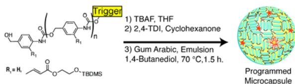
**Figure 3.** Synthesis of microcapsules. The trigger-loaded polymer is treated with TBAF in order to remove the TBDMS protecting group. The free alcohols are then reacted with 2,4-TDI to form a pre-polymer for microcapsule formation. Microcapsules are formed by an interfacial polymerization reaction between isocyanates and 1,4-butanediol.
