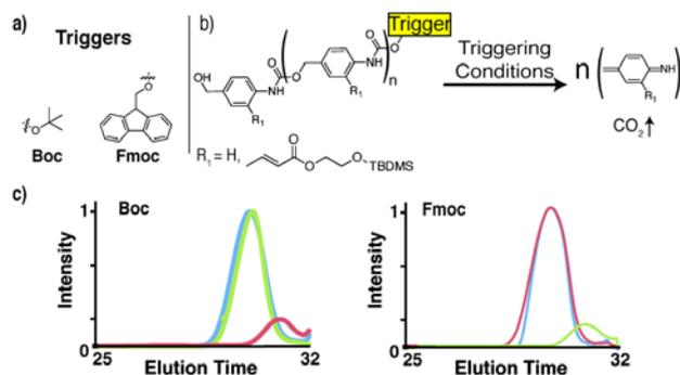
**Figure 2.** Triggered depolymerization of polymers. a) Scheme depicting the polymers and disassembly chemistry. b) GPC traces show disassembly of polymers after removal of trigger. (Green – 10% piperidine, THF, 15 mins), (Red – 1:1 TFA: CH<sub>2</sub>Cl<sub>2</sub> 15 min), (Blue – unexposed Polymer).
