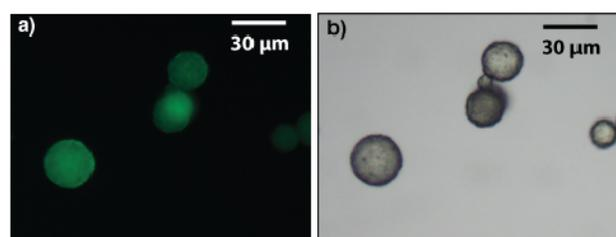
**Figure 4.** Microcapsule morphology. a) Fluorescence microscopy images and b) optical microscopy images of Boc microcapsules (**Boc**). c) SEM image of microcapsule shell-wall.
