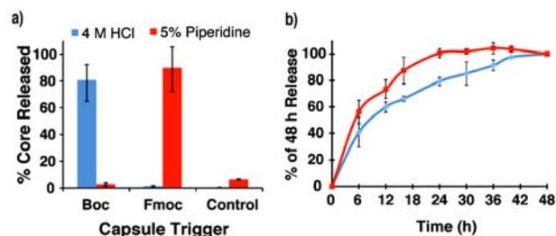
**Figure 5.** Release of core contents. a) Percentage of core released after 48 h in triggering solution for capsule size 5-40 μm. (Blue – 4M aq. HCl w/ 10% EtOH, Red – 5% Piperidine in THF). Percentage of core is calculated as integration of GC peak compared to manual rupture b) Release profile of both triggers (Boc, Fmoc) in their respective triggering solution. The final data point is set as 100% to facilitate interpretation.
