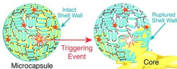
**Figure 1.** Schematic of programmable microcapsules. The capsule shell wall is a self-immolative crosslinked polymer network (blue) with a loaded trigger (star). The capsule releases its content upon activation from a triggering event. This event removes the head of the polymer (star) initiating a head-to-tail depolymerization and release of core contents.
