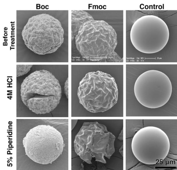
**Figure 6.** Changes in shell-wall morphology. Capsule shell walls are shown before and after 48 h exposure to triggering solutions. Triggered capsules bear a distinct cracking pattern on the outside of their shell wall.
